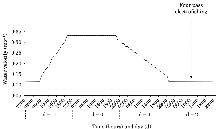
FIG. 1. Average water velocity (measured at 40% of total depth above the bed, every 10 cm, along three transects regularly spaced along each section) of the experimental channel from day d = -1 to day d = 2 , where d = 0 is the day on which the velocity reached its maximum value. The date of the four-pass electrofishing of the channel ( i.e. the end of the experiment) is given.
